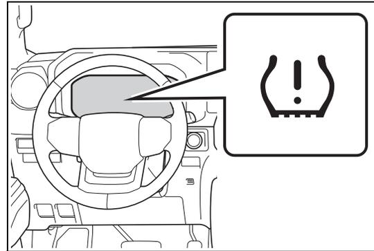
■ **Warning performance of the tire pressure warning system (Setting using the current tire inflation pressure)**
